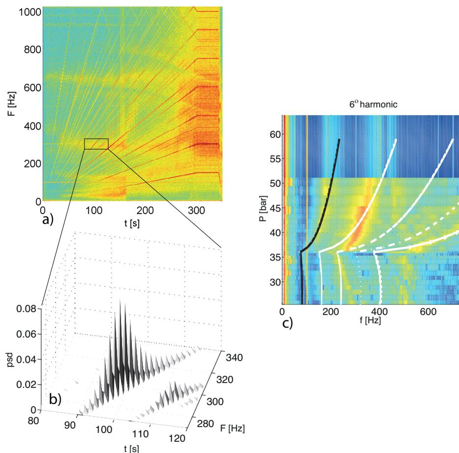
**Figure 1.** a) Spectrogram of the acceleration of the stator. b) Resonant mode of the cavity excited by the turbulent flow. c) Evolution of the resonant mode as a function of pressure and the predicted resonant frequency (black line) and its harmonics (white lines).
