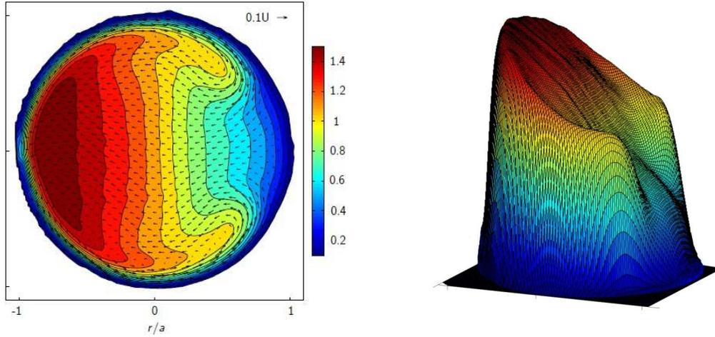
**Figure 2.** Steady and axisymmetric basic flow for  $Re=3600$ . Left: Mean streamwise velocity (color contours) and in-plane velocity (vector field), both normalized with the bulk velocity  $U$ . The maximum velocity arises near the out wall (on the left). Right: Three-dimensional view of the characteristic streamwise velocity profile.
