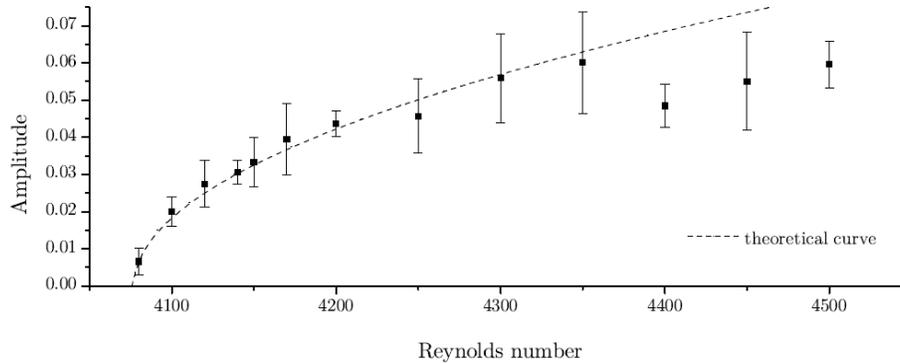
**Figure 4.** Amplitude of the dominant frequency as a function of  $Re$  for  $d/D = 0.049$ . The dashed line is a square root fit to the data. Error bars represent the maximum deviation of the measured values for single revolutions.
