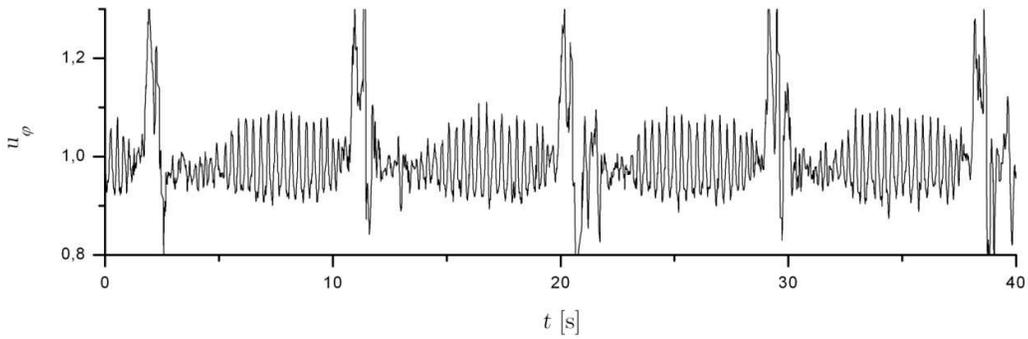
**Figure 3.** Typical time trace of the streamwise velocity for four full revolutions of the sphere in the periodic regime for  $Re > Re_{c,1}$  measured by LDV. The streamwise velocity is periodically modulated between successive passings of the sphere in the vicinity of which the oscillations are interrupted.
