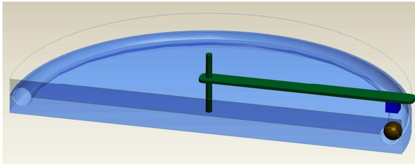
**Figure 1.** Sketch of the experimental setup used to realize a constant flow rate in a torus: two disks of perspex into each of which a concentric notch of half-circular cross sections has been machined, and a rotating boom driving a sphere by means of a magnet. The sphere hence drives the flow.
