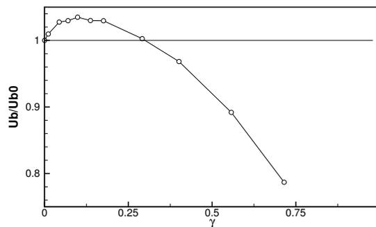
**Figure 1.** Variation of the flow rate  $U_b$  over the uncontrolled value  $U_{b0}$  as a function of the share  $\gamma$  of the available power between pumping power and control power provided to the oscillating walls.
