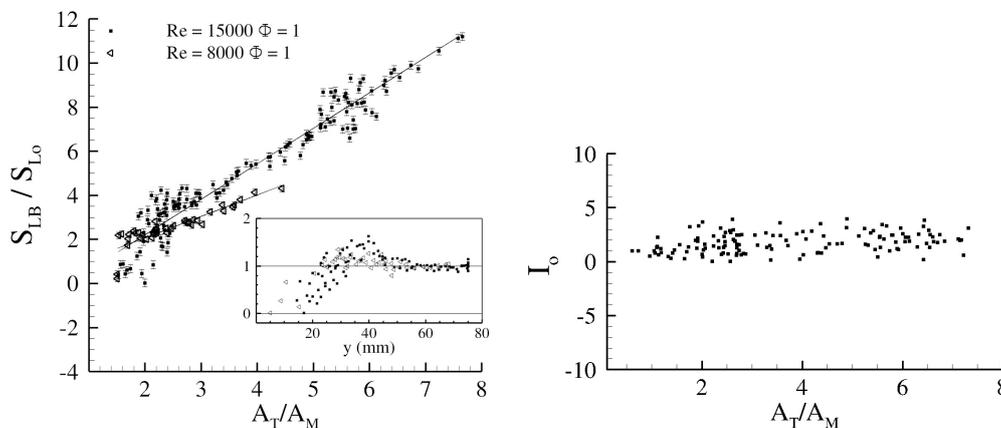
**Figure 1.** Left panel, scatter plot of  $S_{LB}/S_{Lo}$  vs  $A_T/A_M$ . Two best-fits represent values of  $I_o = 0.97$  and  $I_o = 1.61$ . In the inset, compensated plot of  $(S_{LB}/S_{Lo})/I_o$  vs axial coordinate  $y$ . Right panel, scatter plot of  $I_o$  vs  $A_T/A_o$  for a stoichiometric flame at  $Re = 15000$ .
