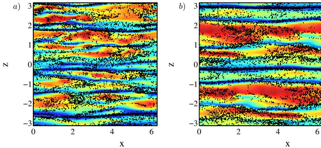
**Figure 1.** Snapshot of an  $x - z$  plane in the buffer layer for a) Newtonian case and b) polymeric flow. Black dots represent particles at  $St^+ = 20$ , and colors indicate the magnitude of the stream-wise velocity component, red being highest and blue lowest.
