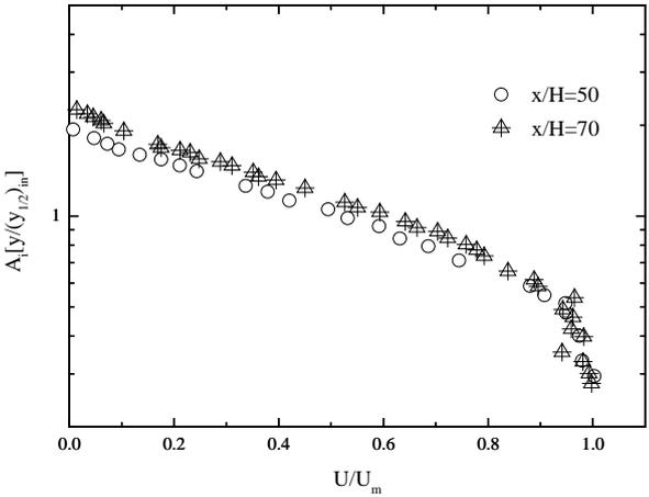
**Figure 3.** The mean velocity profiles on a rough surface in the outer region scaled with the inner length scale.
