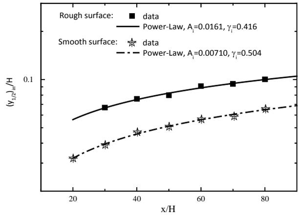
**Figure 1.** The wall jet spread rates in the inner region on smooth and rough surfaces.
