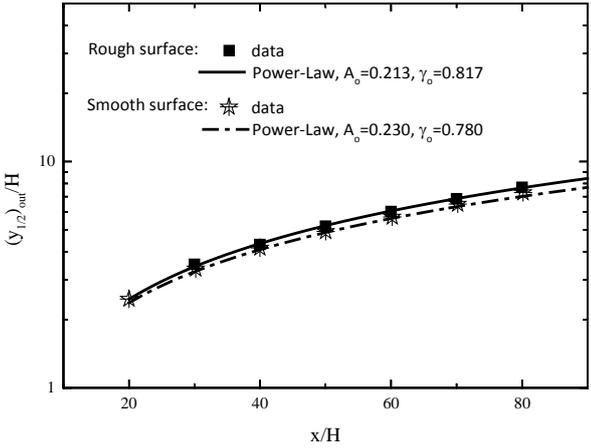
**Figure 2.** The wall jet spread rates in the outer region on smooth and rough surfaces.
