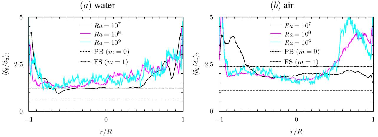
**Figure 2.** Ratio  $\delta_\theta/\delta_u$  of the thermal and viscous boundary layer thicknesses for (a) water and (b) air, as obtained in DNS for different  $Ra$  together with the theoretical estimates for  $m = 0$  (Prandtl–Blasius flow) and  $m = 1$  (stagnation-point flow).
