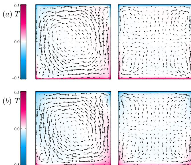
**Figure 1.** Mean temperature distribution in the plane of the large-scale circulation (left) and orthogonal to it (right) in turbulent Rayleigh–B enard convection in a cylinder with aspect ratio diameter/height=1 filled with water ( $Pr = 4.38$ , (a)) and air ( $Pr = 0.786$ , (b)), as obtained in DNS for  $\mathcal{Ra} = 10^8$ .
