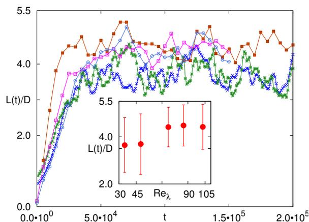
**Figure 2.** Growth of the coarsening length scale,  $L(t)$ , as a function of time and normalized by the Hinze estimate,  $D$ , for  $Re_\lambda \sim 35$  and  $49$  (blue cross and green star),  $Re_\lambda \sim 72$  and  $103$  (purple square and brown filled square), and  $Re_\lambda \sim 86$  (blue circle). Inset: average value of  $L(t)/D$  for different  $Re_\lambda$ .
