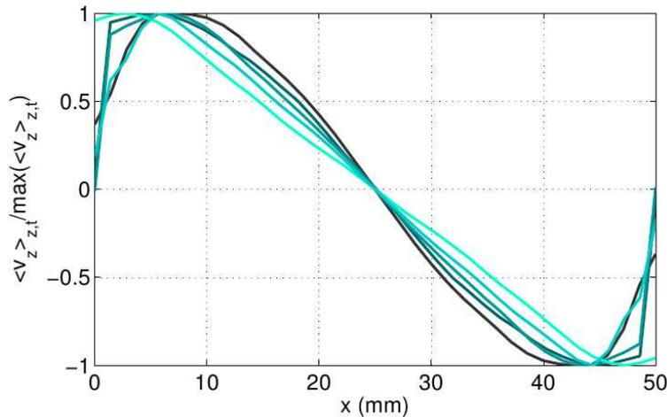
**Figure 1.** The velocity profile, normalized to its maximum, for channel inclination angles of  $0^\circ$ ,  $2^\circ$ ,  $5^\circ$ ,  $10^\circ$  and  $20^\circ$ .
