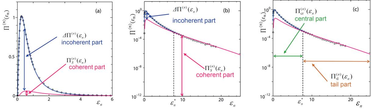
**Figure 1.** Two kinds of divisions of PDF  $\Pi^{(n)}(\varepsilon_n)$ . The division (2) is shown in (a) and (b), respectively, on linear and log scale in the vertical axes. Another division (5) is presented in (c) on log scale.  $\varepsilon_n^*$  is the connection point. The open circles represent an experimental PDF for energy dissipation rates. The contribution of  $\Delta\Pi^{(n)}(\varepsilon_n)$  to the tail part  $\Pi_{\text{tl}}^{(n)}(\varepsilon_n)$  is negligibly small.
