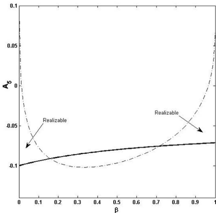
**Figure 1.** Realizable ranges of the  $A_5$  coefficient for linear models, vis-à-vis the psd nature of the M tensor.
