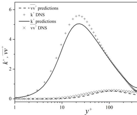
Fig. (1) Comparison between predicted and DNS data for  $k$  and  $\overline{v^2}$
