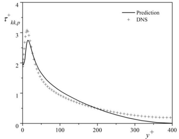
Fig. (2) Comparison between predicted and DNS data for the trace of the polymer stress tensor
