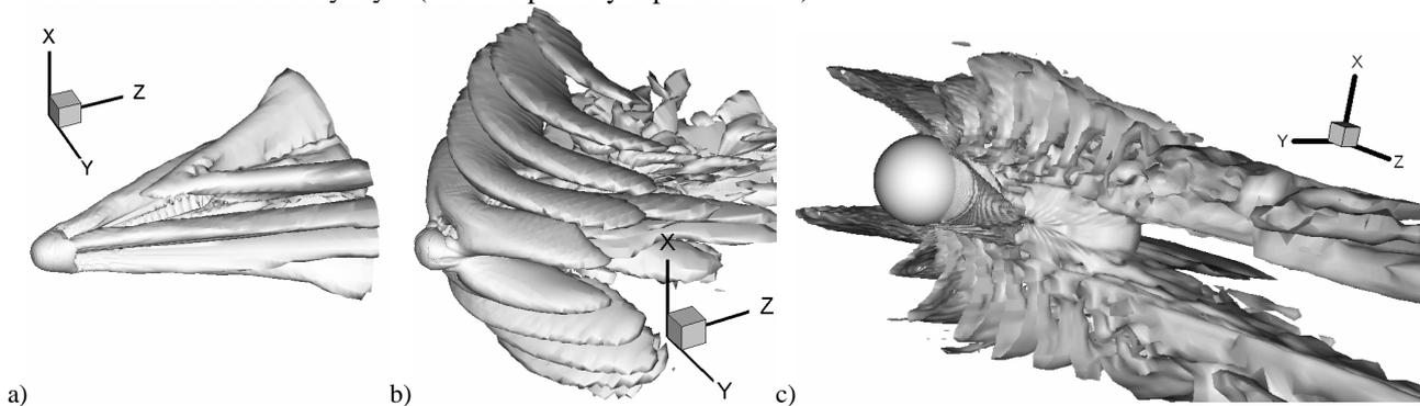
**Figure 1.** Vortex structures of the sphere wake at  $Re = 100$ : a-c –  $Fr = 2; 0.5; 0.08$ ; a-c –  $\beta = 0.005; 0.02; 0.005$ .
