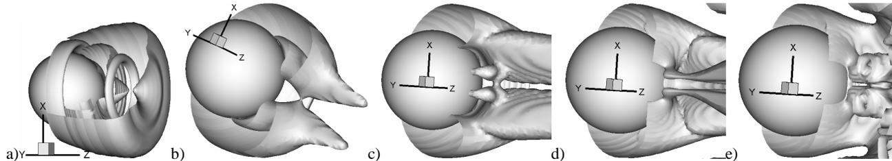
**Figure 2.** The isosurfaces of  $\lambda_2 = -10^{-6}$  &  $-0.16$  at  $Re = 200$  ( $Fr = \infty$ ) (a) and the isosurfaces of  $\beta$  at  $Re = 100$ : b-e –  $Fr = 2, 1, 0.6, 0.35$ ; b-e –  $\beta = 0.15, 0.1, 0.087, 0.087$ .
