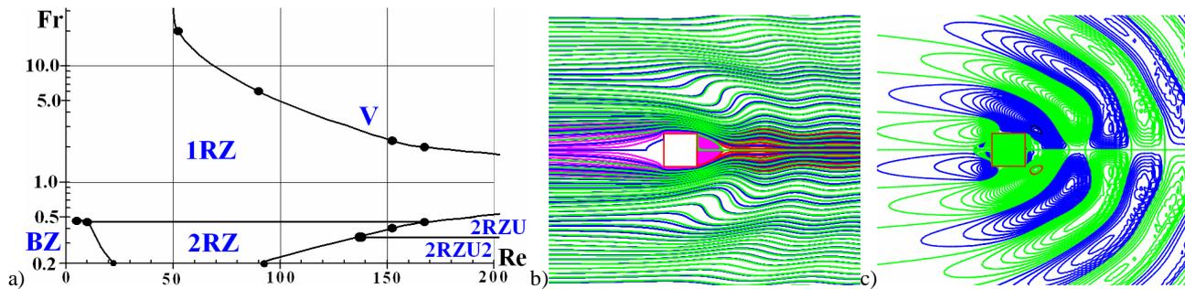
**Figure 3.** The classification of the regimes of 2D stratified viscous fluid flows around a square cylinder (a), stream lines (b) and isolines of  $S_z = \partial p / \partial z$  (c) ( $\delta S_z = 0.227$ ) around a square cylinder at  $Fr = 0.3$ ,  $Re = 50$ ;  $t = 332.07 \cdot T_b$ .
