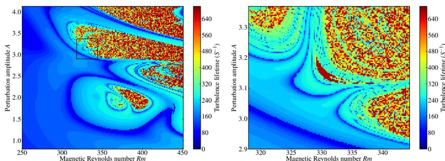
**Figure 1.** Maps of turbulence lifetime as a function of the amplitude of the initial condition  $A$  and  $Rm$  for a given, randomly generated spatial form of initial condition. The right-most figure is a high-resolution map ( $\delta Rm = 0.2$ ,  $\delta A = 0.004$ ) computed for a restricted parameter range (indicated by the black rectangle) of a lower resolution map on the left [13].
