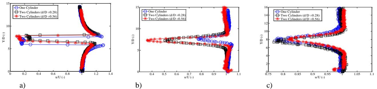
**Figure 4.** Velocity profile. a) Station X/D = 0.1, b) Station X/D = 4, c) Station X/D = 20.
