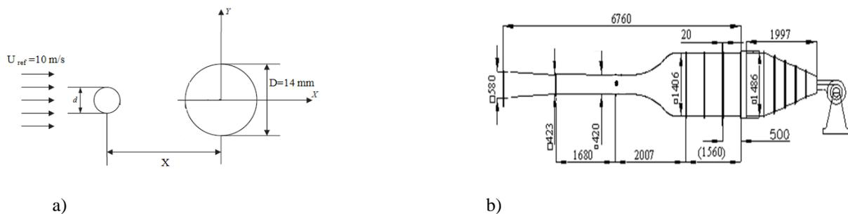
**Figure 2.** Schematic of a) passive flow Over the rod and Circular Cylinder , b) wind tunnel dimension.
