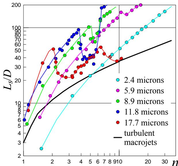
**Figure 1.** Dependence of the length of jet supersonic core on the value of underexpansion for several effective nozzle diameters.
