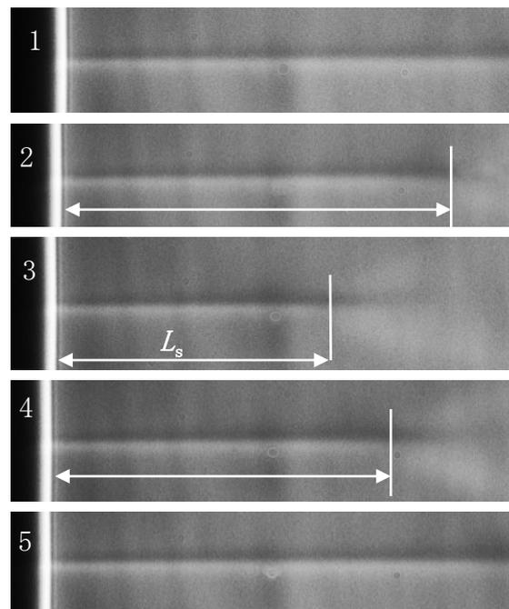
**Figure 1.** Schlieren-visualization of the flow field of microjet outflowing from the nozzle diameter of 35 microns.
