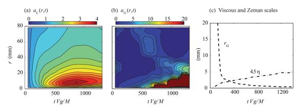
Figure 1. (a,b) Spatio-temporal diagrams showing the ratio of the horizontal-to-vertical energy E (a) and energy flux  $\Pi$  (b) in a decaying turbulence rotating at  $\Omega = 16$  rpm. (c) Time evolution of the Zeman scale  $r_{\Omega}$  and of  $r_{\nu} = 4.5\eta$  which measures the cutoff scale between the transfer and viscous terms of the KHM equation (3) ( $\eta$  is the Kolmogorov scale).
