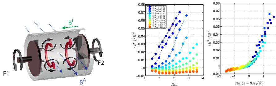
**Figure 1.** (a) Experimental setup of Von Karman Gallium flow. Mean velocity field is represented with full red and black arrows for  $N = 0$ . The directions of applied and induced magnetic field are in dotted blue and green arrows. (b) Evolution of normalized induction with the rotation rate. Each curve is for a different  $B^A$ . (c) Evolution of normalized induction with the non linear correction.
