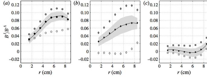
**Figure 2.** Evolution of magnetic profile with  $N$ . (a) Hydrodynamic regime  $N \ll 1$ . (b) Transition regime  $N \sim 0.1$ . (c) MHD regime  $N \sim 1$ . Black curves represent mean profiles and other curves represent the furthest profile from the mean. Grey area shows the rms of the profiles.
