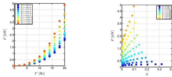
**Figure 3.** (a) Evolution of global injected power with rotation rate. (b) Evolution of global injected power with the interaction parameter. Each color is for a different amplitude of  $B^A$ .
