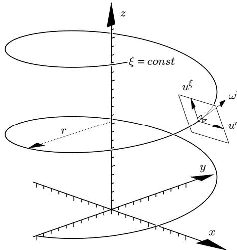
**Figure 2.** Orientation of the helical velocity components and the vorticity in 2D case.
