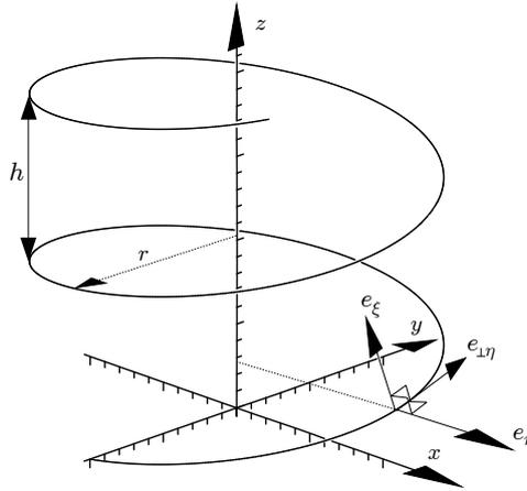
**Figure 1.** Helical coordinates with their respective unit vectors in  $r$ -,  $\xi$  and  $\eta$ -directions.
