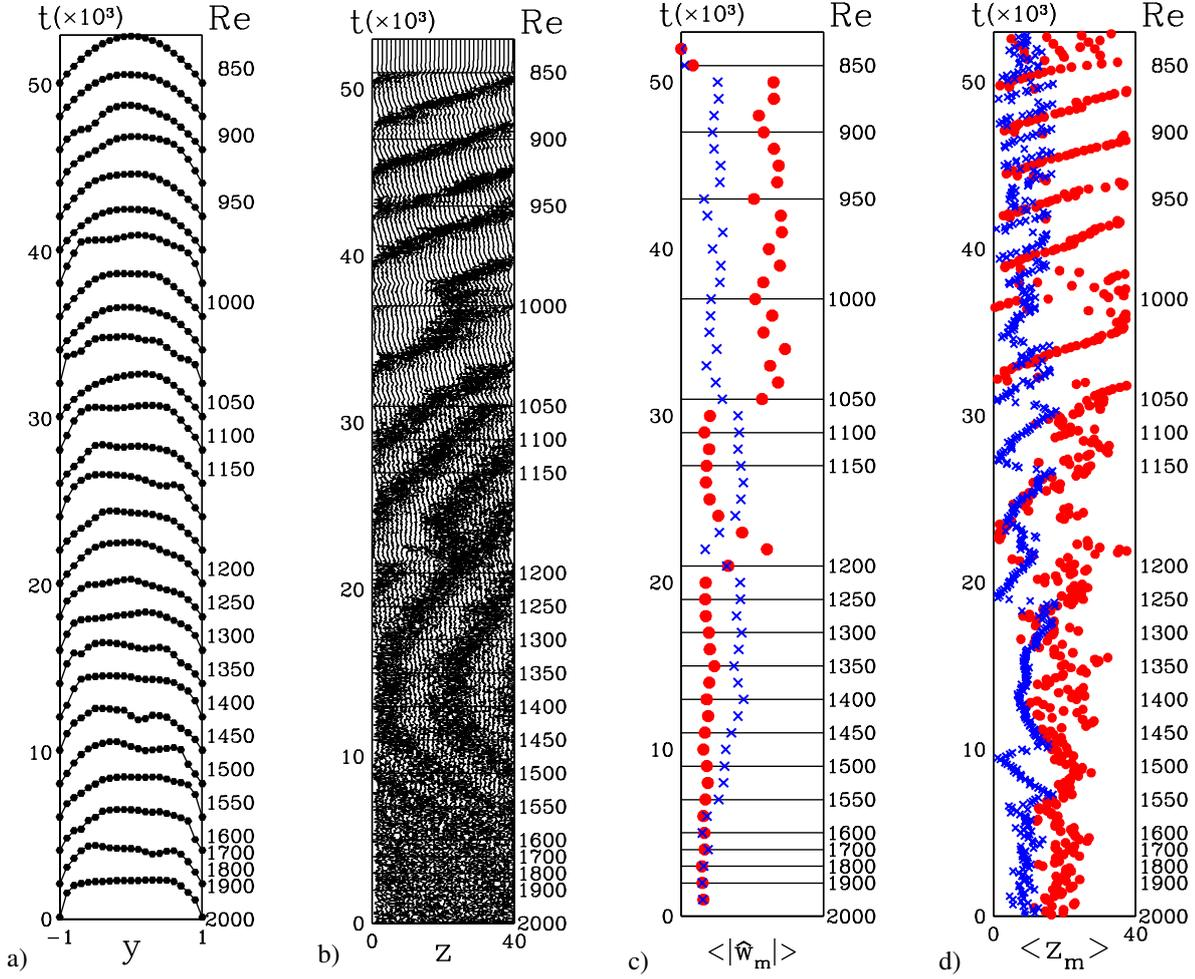
**Figure 1.** Simulation of plane Poiseuille flow in a domain of size  $L_x \times L_y \times L_z = 10 \times 2 \times 40$  in which the  $z$  direction is aligned along the pattern wavevector. The Reynolds number is lowered from 2000 to 850 in discrete steps as indicated along right edge.
