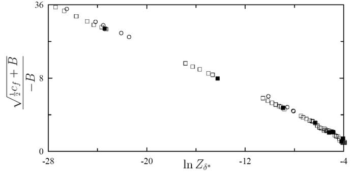
**Figure 2.** Experimental data on skin friction [3, 4] plotted in terms of scaling variables (8);  $\circ$ , [3],  $\square$ , [4] (indirect measurements),  $\blacksquare$ , [4] (measured with floating elements).
