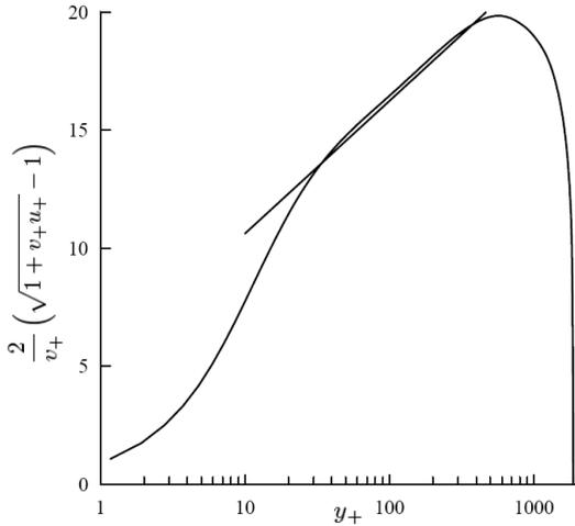
**Figure 1.** Velocity profile near the suction wall in turbulent Poiseuille flow with a constant wall transpiration [2] plotted in similarity variables (5). The straight line has the equation  $\frac{1}{0.41}(\ln y_+ + 2.05)$ .
