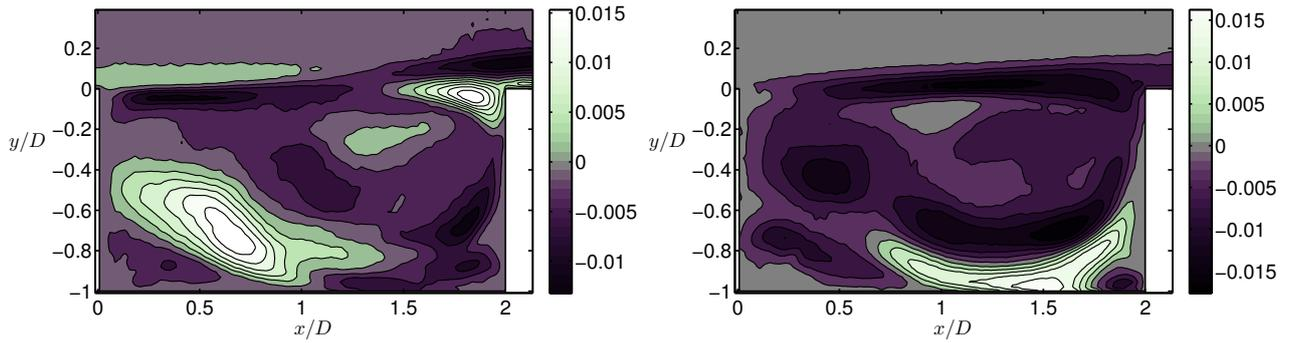
**Figure 2.** Example of global Fourier mode in a  $xy$ -plane, associated with frequency  $f D/U_0 = 0.024$ , for  $Re_D = 4570$ . Real part (left) and imaginary part (right) are depicted with contours of the streamwise velocity  $u'$ , normalised by incoming velocity  $U_0$ .
