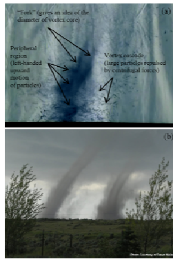
Figure 2. Photographs of vortex structures: (a) typical frame with recorded wall-free non-stationary vortex (negative), 1.68 s after generation, (magnesia particles visualization, the image size is 0.66 by 0.41 m); (b) air tornadoes in northern Lincoln County, Washington (photo by Dawn Nelson, www.wrh.noaa.gov).
