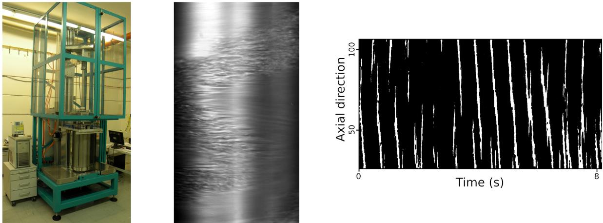
**Figure 1.** *Left:* Picture of the Taylor–Couette experiment. *Middle:* Snapshot of subcritical turbulence for counter-rotating cylinders. *Right:* Space-time diagram of subcritical turbulence. White regions are turbulent, black indicates laminar flow.
