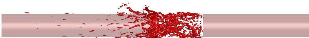
Figure 3. Instantaneous iso-surface of \lambda_2 for L_{\text{gap}} = 2D_{\text{rod}} at t = 108 D_{\text{rod}} / U_{\text{bulk}}
