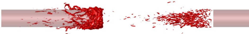
Figure 2. Instantaneous iso-surface of \lambda_2 for L_{\text{gap}} = 6D_{\text{rod}} at t = 108 D_{\text{rod}} / U_{\text{bulk}}
