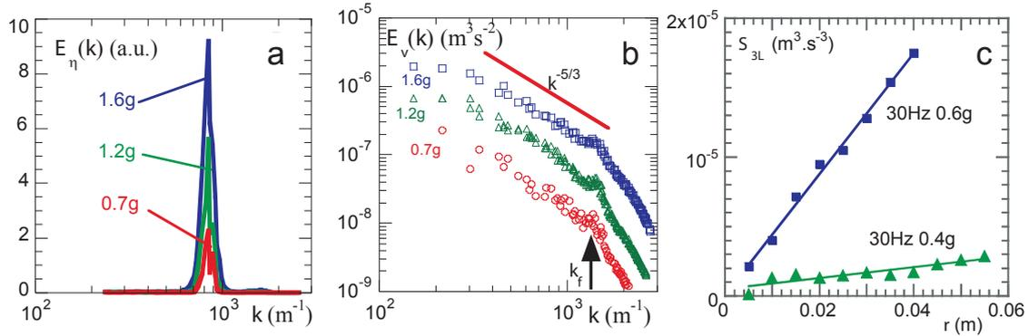
**Figure 2.** Wave number spectra of the surface elevation (a), and of the kinetic energy of the horizontal flow (b) at different levels of the vertical acceleration ( $a = 0.7$  g,  $1.2$  g, and  $1.6$  g) and  $f_0 = 60$  Hz. (c) Third moment of the longitudinal velocity increments in the surface ripple driven turbulence at  $f_0 = 30$  Hz and at ( $a=0.4g, 0.6g$ ).
