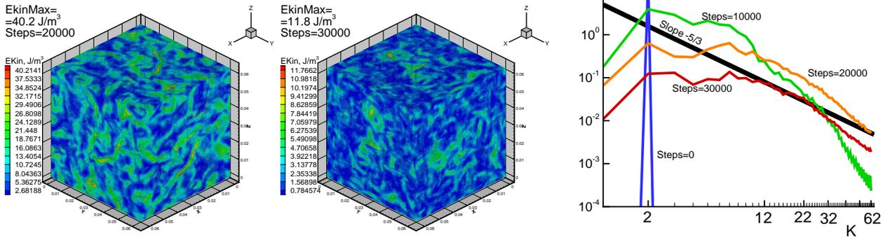
Figure 2. Time-evolution of kinetic energy and spectrum
