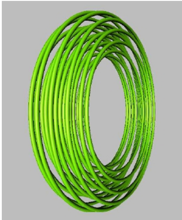
Figure 1. Example of laminar bundle of vortex rings (note that the thickness of each constituent vortex ring is for the sake of visualization only, as the radius of the vortex core is infinitesimal).
